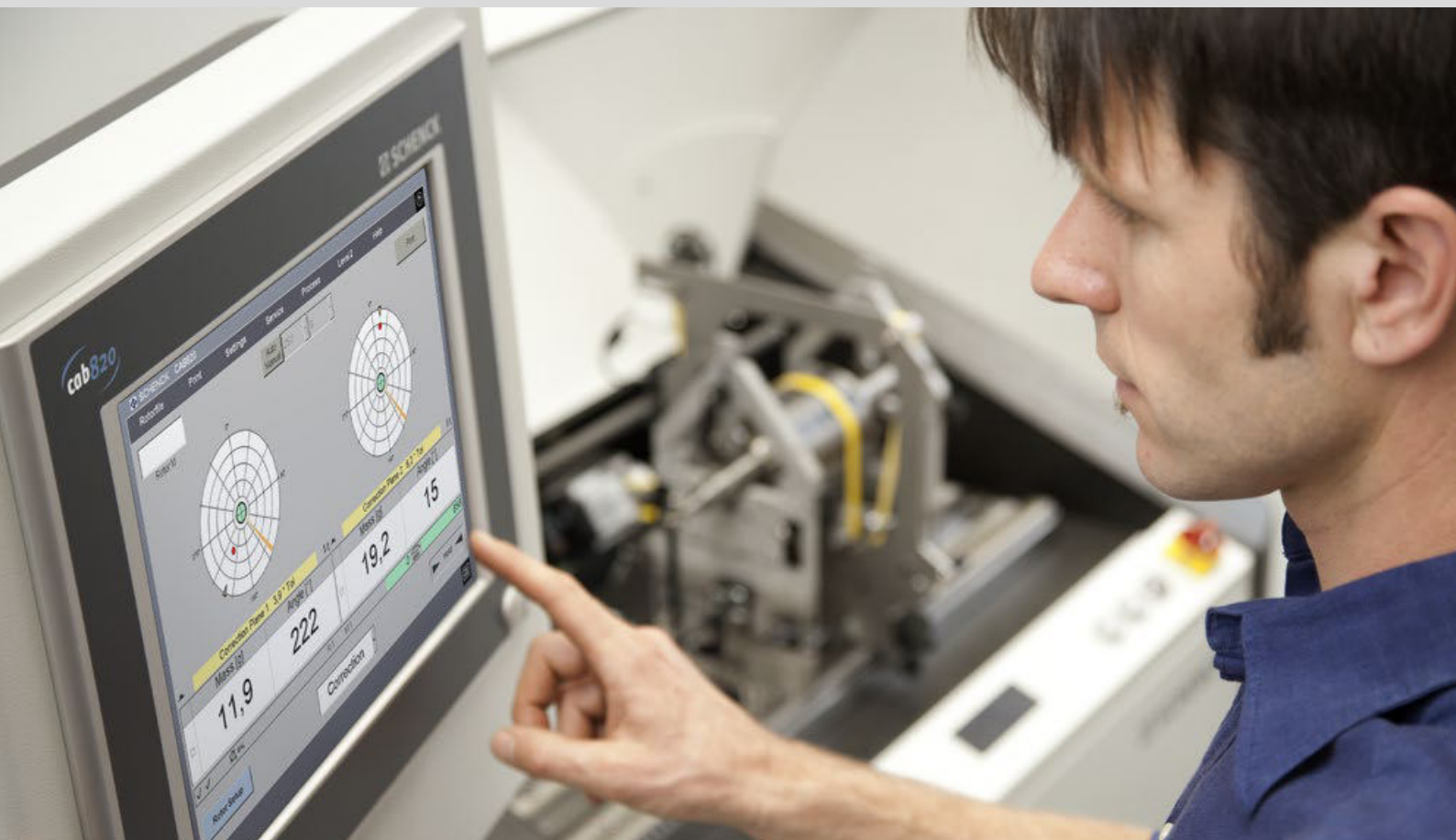
Convenient touch-screen operation of all CAB measuring units
