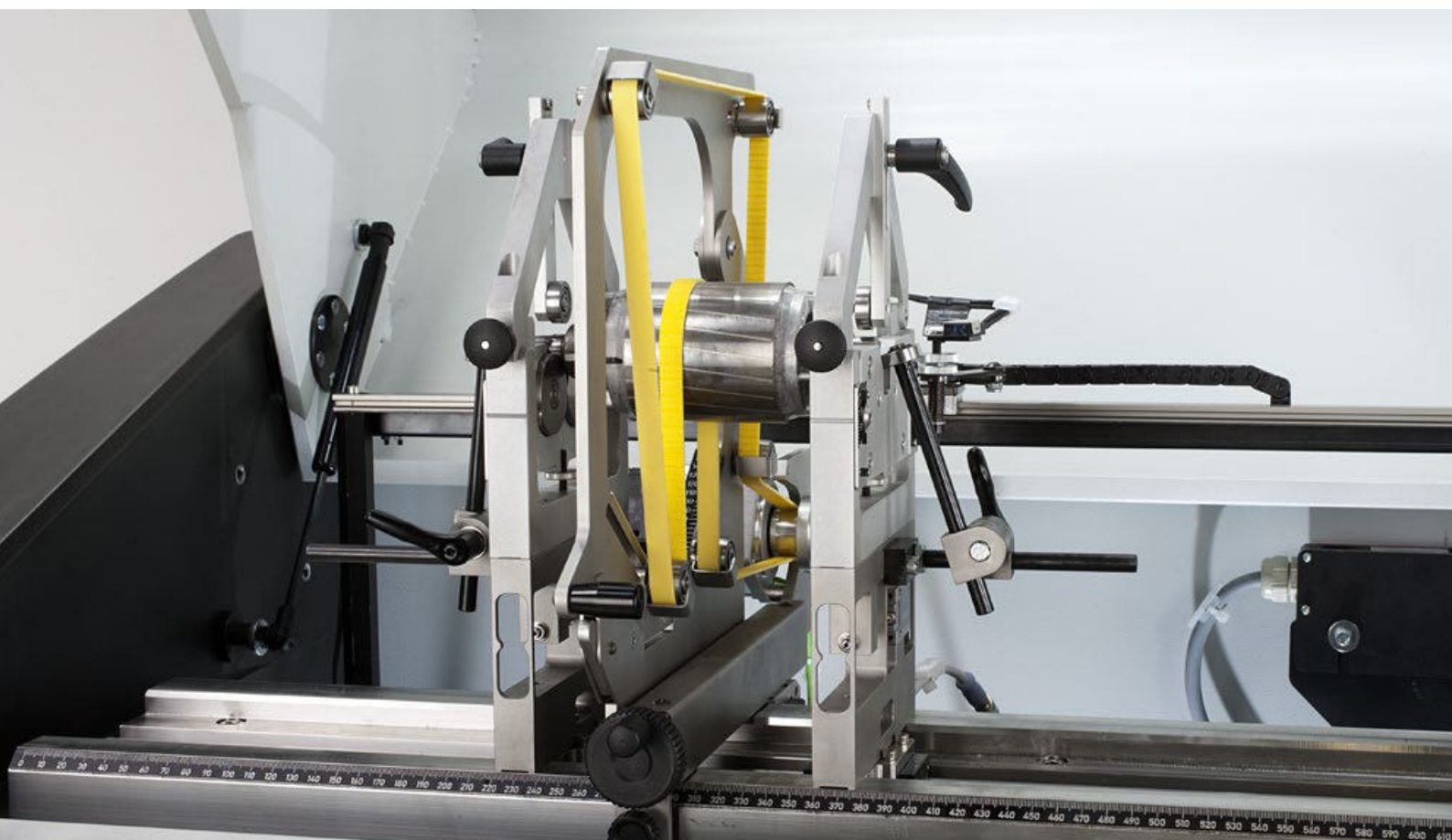
Non-Magnetic design of all components in the test space
