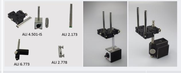
Single parts (left); magnetic foot holder for sensor assembled for surface measurement (center) and point scanning (right)
