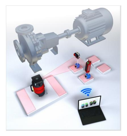
GEO CENTER communicates directly with the measuring components via Bluetooth.
